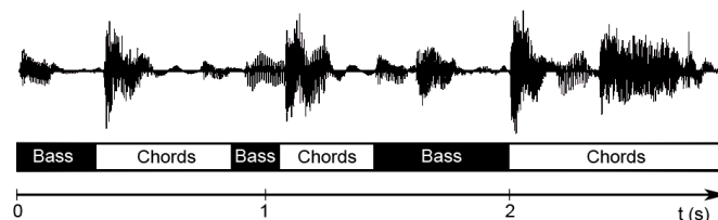
Fig. 5. Identification of bass and chord parts in a Bossa nova guitar audio signal
