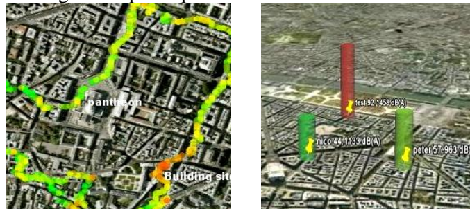
Fig. 3 – Visualisation with Google Earth. On the left, the collective noise map generated by all the measures. On the right, a real time visualization of the collective noise exposure.
