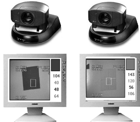
Figure 2: Two Talking Head cameras and associated monitors showing what each camera perceives.
