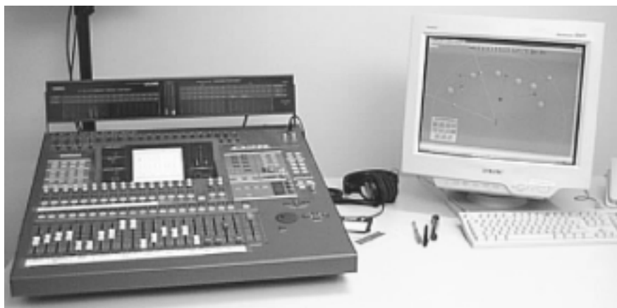
Figure 8: the MusicSpace system connected to a mixing console
