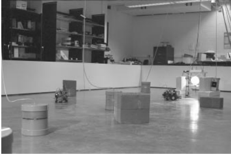
Figure 1: Physical robots used in the experiments. The robot has on-board computational resources, a battery, left and right motors, and about 30 sensors, including vision. The robot “lives” in a robotic ecosystem together with other robots. There is a charging station as well as competition for the available energy.
